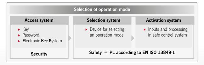
The access system does not have to be implemented according to EN ISO 13849-1. It is not possible to determine a PL for the monitoring of an authorization. By contrast, the selection system and the safe control system of a machine must fulfill the required PL. This is very simple for mechanical controls or key-operated rotary switches.
