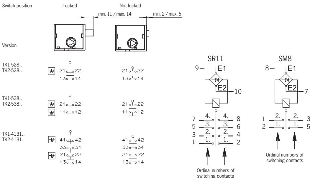
Figure 2: Switching elements and switching functions
