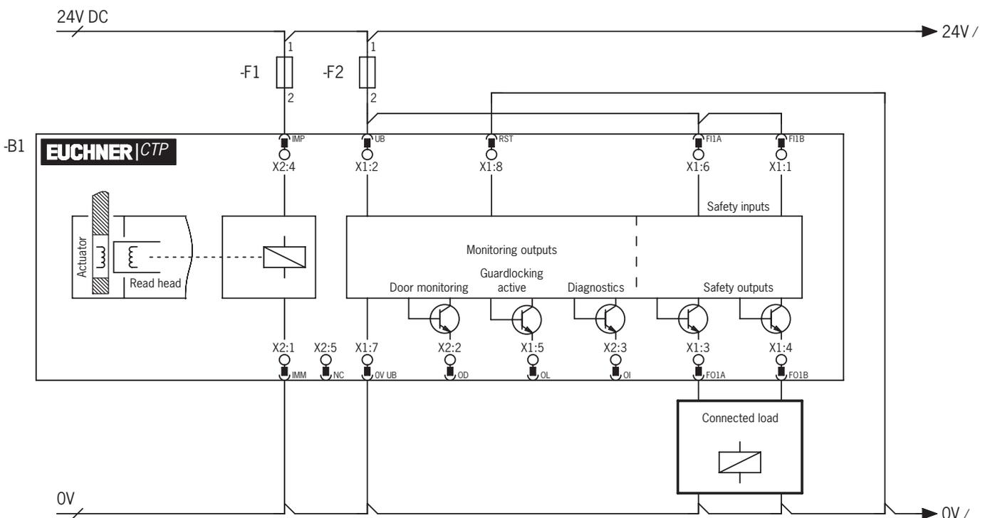
Figure 4: Connection example for separate operation, version with plug connectors 2xM12
