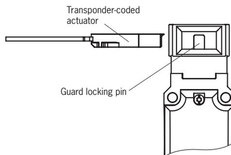
When the guard is closed, the actuator is moved into the safety switch. When the switch-on distance is reached, power is supplied to the actuator by the switch and data are transferred.
