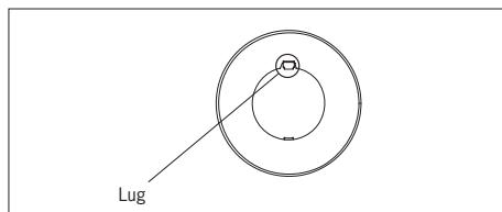
Break off the lug on the rating plate using pliers before installing the rating plate.
